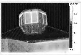
Conversely, the above traditional structure is experiencing intense heat loss through the rooftop window assembly while letting in less light.
