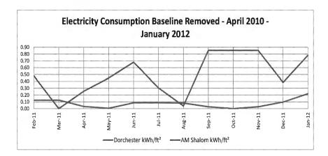
The above graph illustrates electricity consumption per square foot for both structures. Baseline data has been removed to isolate consumption attributed to outdoor weather conditions. Consumption is considerably higher in the traditional structure. Electricity usage is consistent throughout the Sprung facility.
