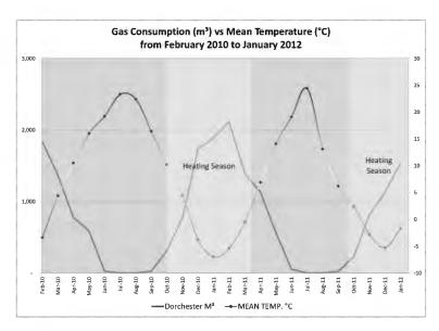
Above, displays natural gas consumption relative to average outdoor temperature. An increase in consumption during the winter months is attributed to gas-fired heating equipment. Consumption does not occur during the summer months.
