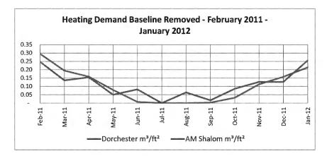
Above, shows natural gas consumption (per square foot) for both structures. Baseline data has been removed to isolate consumption attributed to outdoor weather conditions. Consumption is similar in most building during the winter months; however, the traditional structure uses gas-fired equipment throughout the year resulting in higher annual values.
