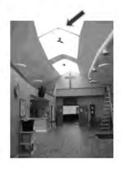
Above, the Sprung structure allows sunlight though a semi-translucent panel section, running the length of the building. MMC uses semi-translucent membrane panels that allow natural daylight into the facility without having the heat loss associated with glazing and framing, shown in the second image.
