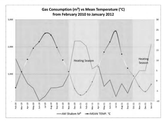
The following graph displays natural gas consumption relative to average outdoor temperature. Consumption appears to increase during the winter months, indicating heating is provided by gas-fired equipment. Low levels of consumption during the summer months indicate a gas-fired water heater.
