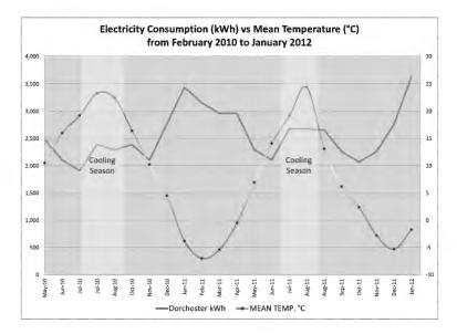
The above graph displays electricity consumption relative to average outdoor temperature. An increase in consumption is evident during the summer months, indicating an electric air conditioning unit. Additionally, spikes in consumption that occur during the winter months can be attributed to electric space heaters.
